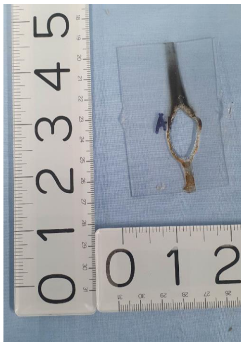
Cavity switch thermoplastic sample 1 after needle flame test
