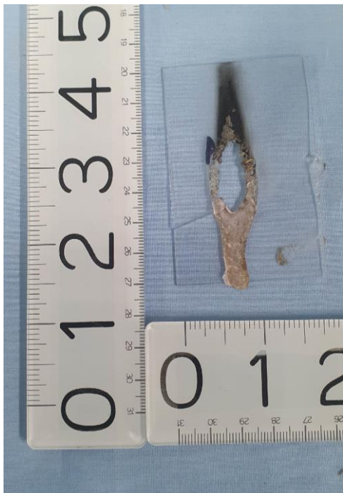
Cavity switch thermoplastic sample 2 after needle flame test
